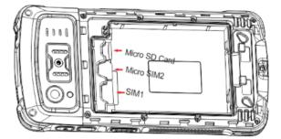
Step 1: Slide the battery cover latch to the unlock position and remove the cover.
