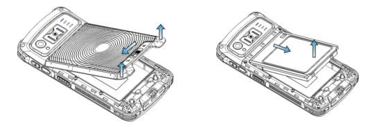
Step 1: Hold down the Power key for 5 seconds and then tap "Power off" to turn off the terminal. Slide the battery cover latch to the unlock position and remove the cover.
