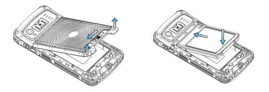
Step 1: Slide the battery cover latch to the unlock position and remove the cover.
